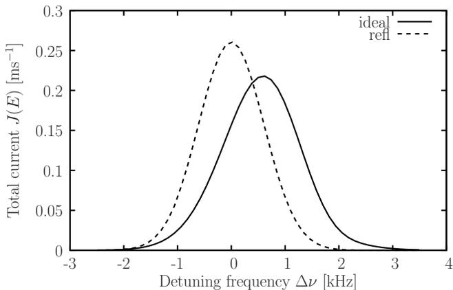
FIG. 1: Total current (per atom) as a function of radio frequency detuning  $\Delta\nu = E/\hbar$  from eq. (29) (for the sign of the detuning see the endnote [30]). Also shown is the reflection approximation (dashed line). The area underneath the curves is fixed by the sum rule (19). Parameter:  $a = 0.4 \mu\text{m}$ ,  $\gamma/\hbar = 100 \text{ Hz}$ ,  $F = m_{\text{Rb}} g$ , with  $g = 9.81 \text{ m/s}^2$ , and  $m_{\text{Rb}} = 87 \text{ u}$ .
