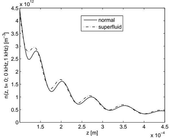
FIG. 8: Density profile of the fermionic beam outcoupled with two different RF  $|E_{\text{grav}} - E_{\text{trap}}|/h$  and  $1\text{kHz} + (E_{\text{grav}} + E_{\text{trap}})/h$ . We show the density profile (eq. (73)) at the center of the beam for a Fermi gas with  $N = 70$ ,  $\omega_z = 2\pi 1.2$  kHz,  $\omega_{\perp} = 2\pi 120$  kHz, and pairing gap  $\Delta = 3.36$  kHz,  $\gamma/h = 100\text{Hz}$ ,  $m_K = 40$  u.
